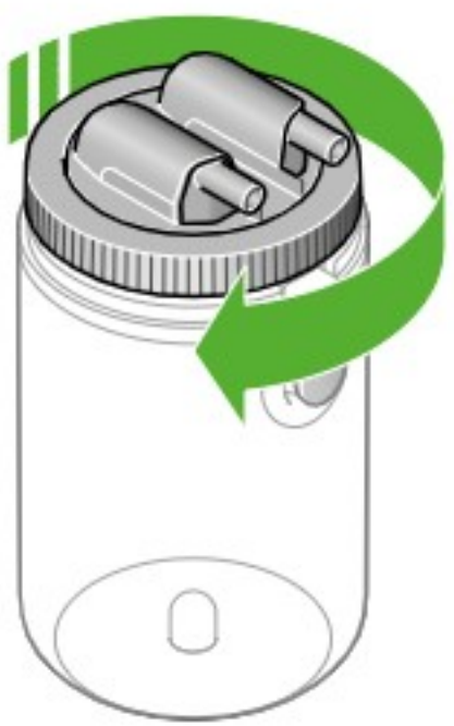
Diagram showing how to reassemble the Dirty water tank.
